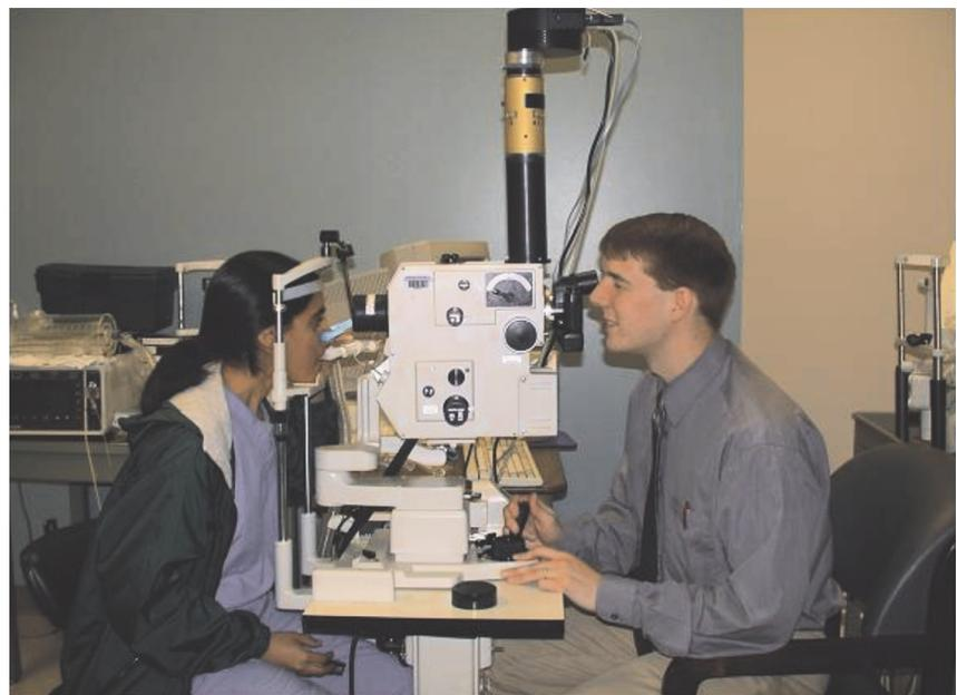
Figure 6. The oximeter was mounted on the Polaroid port of a Topcon 50VT camera. The black cylinder attached to the camera is a 2X lens. The gold cylinder immediately above is the image splitter and bandpass filters. The black digital camera on top is used to quantify light at the various frequencies
